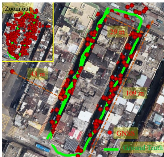
Fig. 14. Experiment 2: Trajectory of the vehicle is indicated by green curve. The red circles indicate the object detection aided GNSS positioning results.
